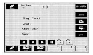
The numbered screen buttons, 1 through 6, represent the order of the discs loaded in the changer. If there are only two discs loaded, only screen buttons 1 and 2 will be available.
